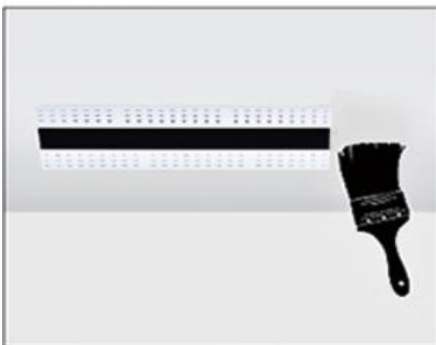
4. Do dusting (painting) at the side of Embedded parts
