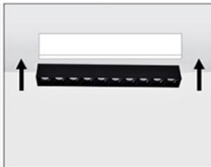
5. Connect 220V wire with LED driver, Then push light body into embedded part
